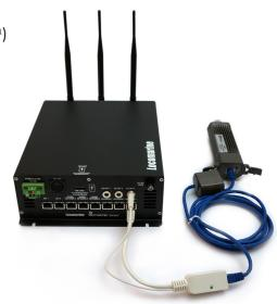
Yacht Router Standard is equipped with Vessel-to-Shore WIFI Booster for simple installation and zero coax cable signal loss. WIFI Booster is powered directly from Yacht Router via Power-over-Ethernet cable injector.
